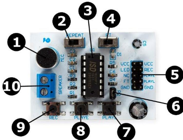
1. **MIC** – Microphone input. The microphone input transfers its signals to the on-chip amplifier.
