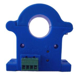
The WBI222LX05-25 is is a split core hall effect sensor for the measurement of AC/DC current with standard voltage output  $0\sim5(10)$ V.The product has certain advantages of total galvanic isolation between input/output, high accuracy, low drifting by temperature, and wide temperature bearable range, etc.
