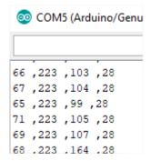
The first row is AINO, connected to the photodiode (if the jumper is set). Change the light intensity and you will see the value changing. The third row is "floating" as nothing is connected to AIN2.
