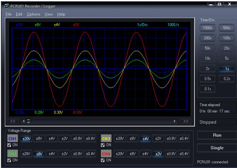
Using this screen the 4 channels can be viewed simultaneously as a trace on the screen
