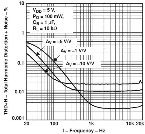
Figure 6. Total Harmonic Distortion + Noise vs Frequency
