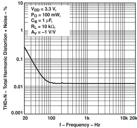
Figure 5. Total Harmonic Distortion + Noise vs Frequency
