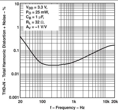
Figure 1. Total Harmonic Distortion + Noise vs Frequency
