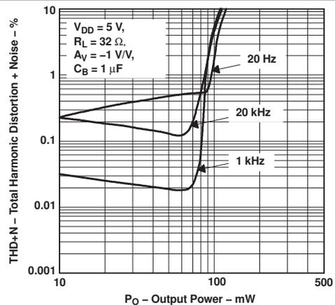
Figure 4. Total Harmonic Distortion + Noise vs Output Power
