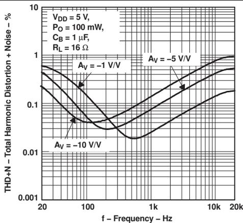
Figure 13. Total Harmonic Distortion + Noise vs Frequency
