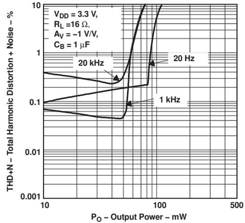
Figure 12. Total Harmonic Distortion + Noise vs Output Power
