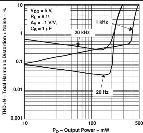
Figure 10. Total Harmonic Distortion + Noise vs Output Power
