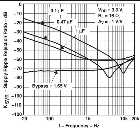
Figure 15. Supply Ripple Rejection Ratio vs Frequency
