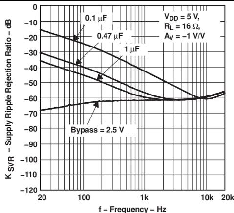
Figure 16. Supply Ripple Rejection Ratio vs Frequency
