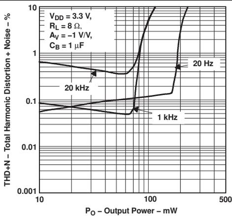
Figure 8. Total Harmonic Distortion + Noise vs Output Power
