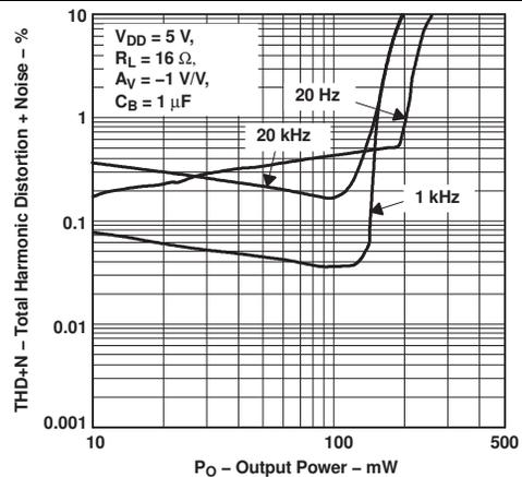
Figure 14. Total Harmonic Distortion + Noise vs Output Power
