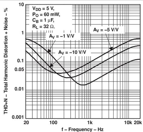
Figure 3. Total Harmonic Distortion + Noise vs Frequency
