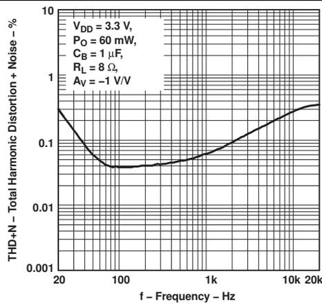
Figure 7. Total Harmonic Distortion + Noise vs Frequency
