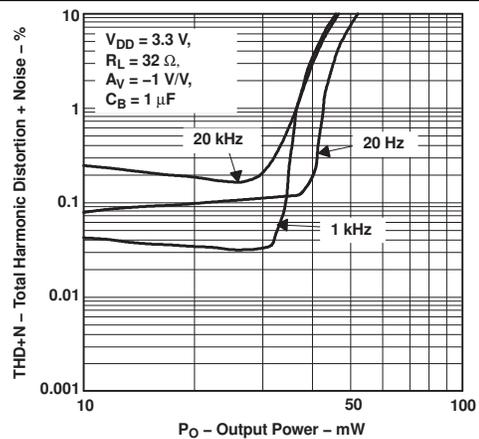
Figure 2. Total Harmonic Distortion + Noise vs Output Power
