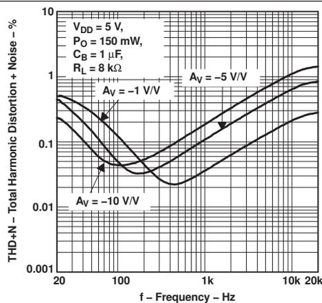
Figure 9. Total Harmonic Distortion + Noise vs Frequency
