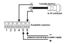
Figure 01 - Connections of theTxConfig Interface - Loop powered or power supply
