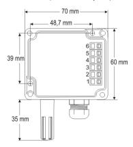
Figure 06 - TEMP/WM fixing holes and housing dimensions.
