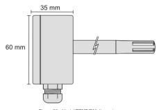
Figure 05 - Model TEMP/DM dimensions
