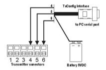
Figure 02 – Connections of theTxConfig Interface - 9 Vdc battery power
