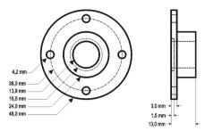
Figure 04 - Mounting flange for TEMP-DM.
