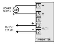
Figure 08 – 0-10 VDC connections
