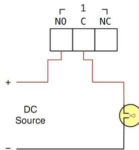
**Figure 8 - Wiring a basic DC load**
