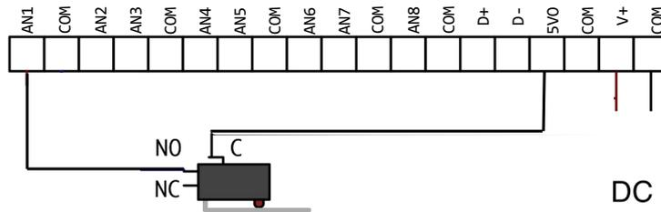
Figure 3 - Wiring a dry contact switch
