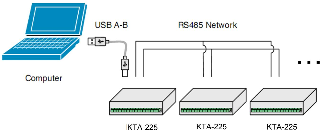
**Figure 1 - Connecting multiple controllers with a RS-485 network**
