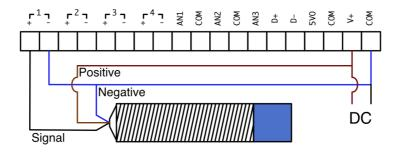
Figure 5 - Wiring a PNP-type sensor
