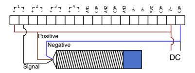
Figure 4 - Wiring an NPN-type sensor
