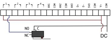
Figure 3 - Wiring a dry contact switch
