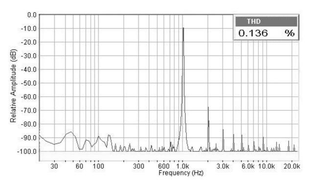
Harmonic Distortion at 1 kHz. 100 mW into 8 ohms. 12V DC input from battery.
