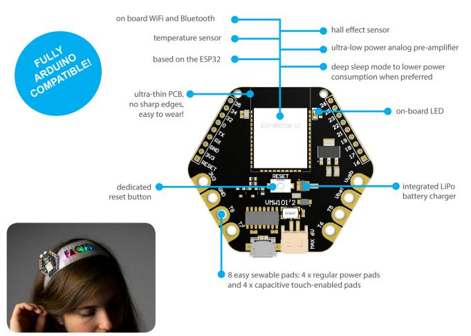
Get ready to meet the most versatile wearable and ESP32 based development board of the moment! It's 100% Arduino compatible and it's easy to wear thanks to its uniquely thin PCB with 8 x sewable pads.
