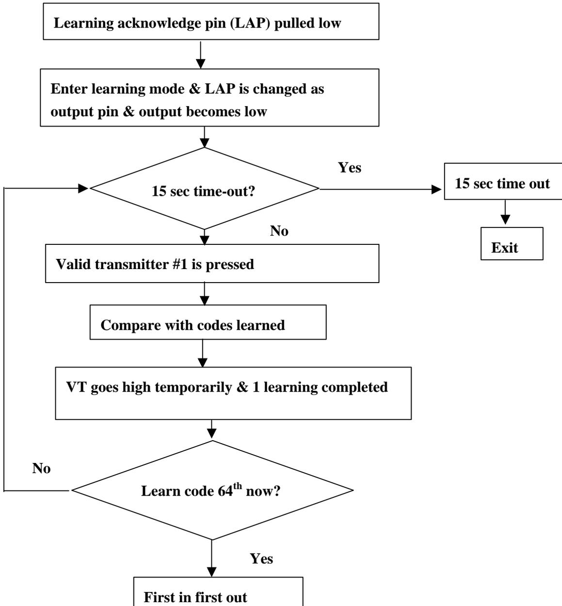
If 15 seconds of period is not long enough for learning all the transmitters, then the 2nd or the 3rd cycle of learning can be done until all the transmitters (up to 15 or 31 or 63 or 127 or 225 depending on which model of RX-3302D) is learned.
