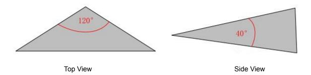
Place the product into a predetermined position, and when someone enters the sensitive area, it automatically plays back the sound. The sensor can be rotated 60 ° both leftward and rightward, so users can turn it to different sensing areas according to the actual needs.
