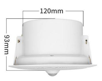
Note: The diameter of the hole for mounting on the ceiling is 160-170mm.
