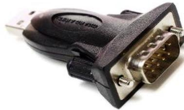
Figure 2: USB to RS232 converter
