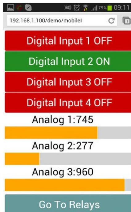
The KTA-323 custom Arduino sketch contains code for serving out a web page as well as a mobile optimised version. The web server listens for HTTP requests on port 80, and serves out the configuration page when requested.
