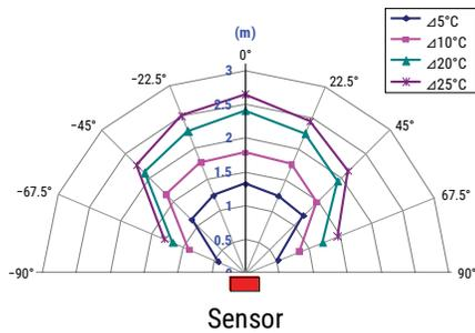
$\Delta T$  (°C) = Difference between room temperature and heat source temperature
