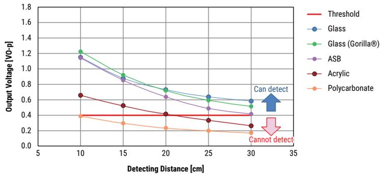
Measuring conditions: Transfer velocity - 1 m/s
