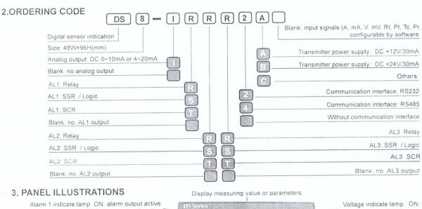
Alarm 1 indicate lamp ON: alarm output active OFF: alarm output inactive Alarm 2 indicate lamp ON: alarm output active OFF: alarm output inactive Alarm 2 indicate lamp ON alarm output active OFF: alarm output inactive OFF: alarm output inactive Display parameters value or input ratio
