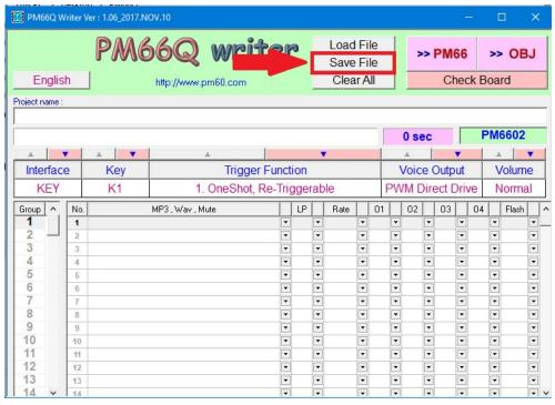
Step 10: After clicking the "Save File" You can proceed to click the "PM66" button as seen below to put your sound onto the sound module. After this step, you can disconnect the sound module from your computer and add the batteries. The unit should play your sound when the corresponding button is pressed.
