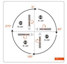
After took the twenty second point, again rotate 90°horizontally, alternate the positive Roll value R=+55
