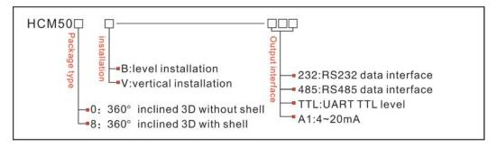
E.g: HCM508B-232: 360tilt 3D sealed with enclosure /RS232 output
