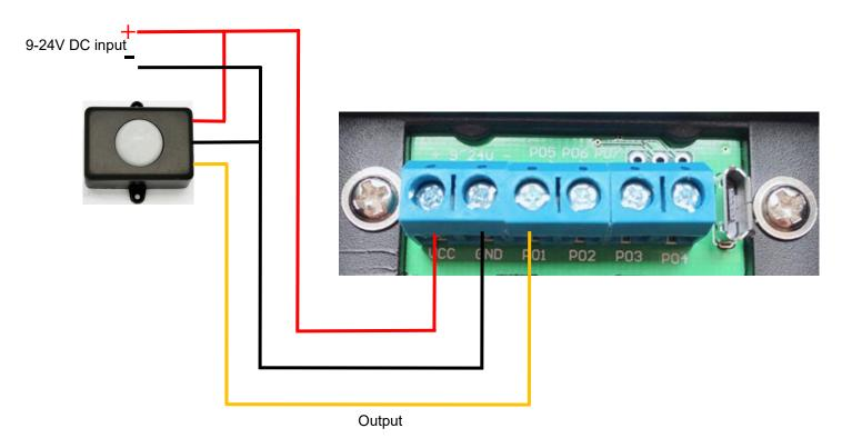
This wiring method is for those customers' reference, who need the player to be triggered by a PIR sensor. Besides, to achieve this function the trigger mode in the configuration file must be "2". When the PIR sensor and the player share the same power source, please make sure the PIR sensor is allowed to work at the same voltage with the player.
