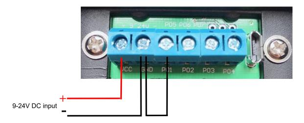
This wiring method is for those customers' reference, who need the player to play the sound messages automatically in a loop once it's powered up. Besides, to achieve this function the trigger mode in the configuration file must be "3".
