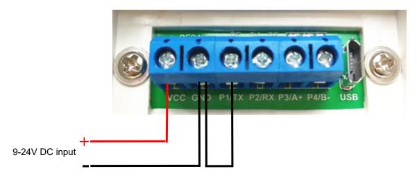
This wiring method is for those customers' reference, who need the player to play the sound messages automatically in a loop once it's powered up. Besides, to achieve this function the trigger mode in the configuration file must be "3".
