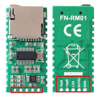
In order to connect to external buttons easily based on AD key control for users to accomplish button control, we made the solder pads at the bottom of the module as shown above marked with the red box. Through AD key function(the solder pad "KEY") and connecting with specific values of resistors, users can lead out 5 different functional key control as below. Please refer to the application circuit 5.1 for the connection in details of this part.
