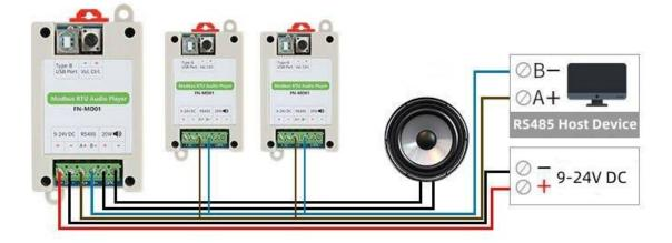
This example is only one of the wiring methods. This device is widely used, and the wiring method may be different in different application scenarios. The working voltage range of this product is 9-24V DC, so please do not exceed the voltage range, so as not to cause the device to burn.
