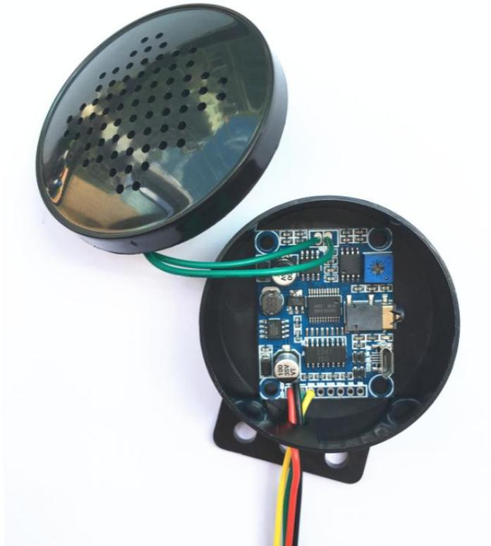
2). And pick up the top cover / speaker, then you will see it shown as the picture below. See the micro USB port and the volume potentiometer on the audio player board.
