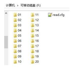
2). Put the audio files in each folder, which can contain maximum 255 audio files. Each folder must contain all Mp3 **OR** Wav audio files. Mp3 and Wav cannot co-exist within each folder. Rename them "001.mp3/wav" to "255.mp3/wav" as shown below. For the quickest timely response once triggered; we suggest that no more than audio files in each folder.
