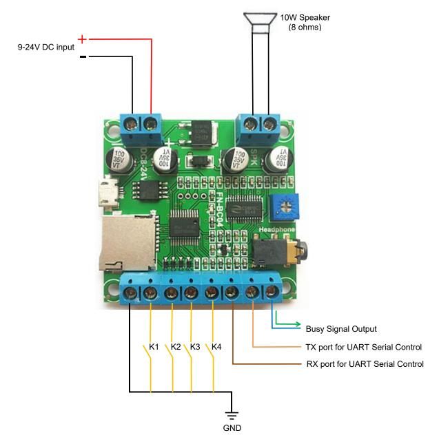
Notes: 1). The Busy port outputs a signal in low level when the module is playing a sound, and it output a signal in high level when the module is standby.
