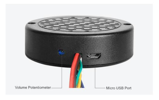
As you can see the picture above, there is a micro USB port, and you can connect it to computer through an Android phone purposed USB data cable to load audio files and configuration file. Once the connection is done, the internal flash memory will be detected and displayed on PC working as a USB flash drive.
