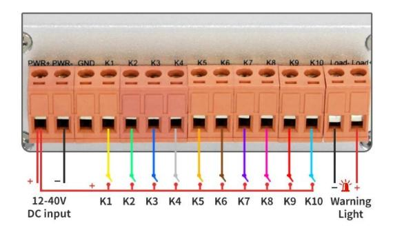
Note: The negative trigger version also can be activated with a low level signal (0V) while the positive trigger version can be activated from a high level signal (12-40V) from a PLC or controller. The PLC or controller needs to share the same ground with the player in advance.
