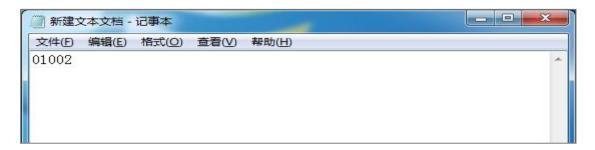
There is a 5-digit value in the config file. The 1<sup>st</sup> digit represents the function of the buttons; the 2<sup>nd</sup> and 3rd digits represent the volume setting; the 4<sup>th</sup> and 5<sup>th</sup> digits are the device address. Let's take "01002" as an example to further explain as below.
