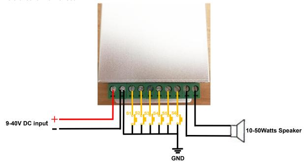
Note: When connecting with a 50watts speaker, 24V power supply is the minimum and the output current cannot be less than 2000mA.
