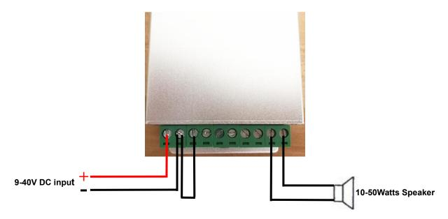
This wiring method is for those customers' reference, who need the player to play the sound messages automatically in a loop once it's powered up. Besides, to achieve this function the trigger mode in the configuration file must be "4" for the first trigger input only.
