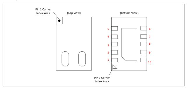
**Pin Diagram:** The Exposed Pad is underneath
