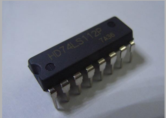
Figure 2: Flip Flop IC (DIP 16 package)
