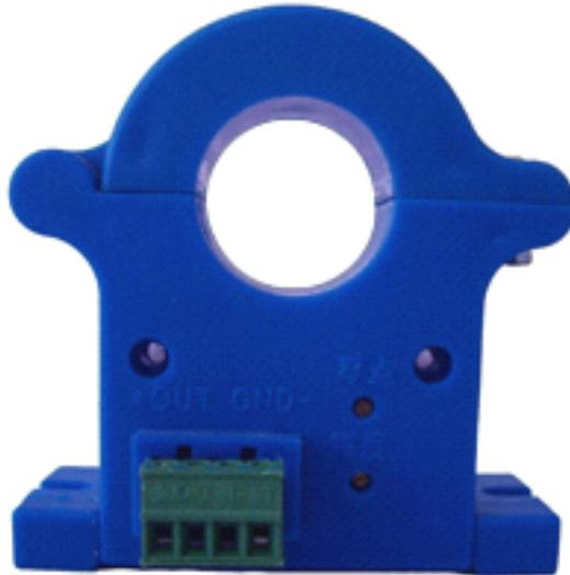
The WBI222LX05-25 is a split core hall effect sensor for the measurement of AC/DC current with standard voltage output 0~5(10)V. The product has certain advantages of total galvanic isolation between input/output, high accuracy, low drifting by temperature, and wide temperature bearable range, etc.
