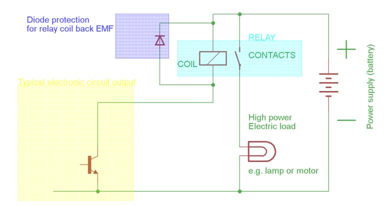
An interesting characteristic of a relay coil is that the coil will "store energy" in the inductance of the coil when the coil is switched on (energised). When the relay is switched off, this energy is released as an Electromotive force (EMF) that generate a voltage pulse in the opposite direction as the original applied voltage. The diode will "short circuit" the current and stop the generation of a high voltage pulse that can damage the electronic device.
