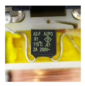
The AC signal will first see a thermal cutoff IC used to protect the supply if there is a large load attached that draws too much current. This is a nice added level of protection that is not found in all wall-warts, just the nice ones.
