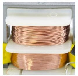
Next, you have a single phase, shell-type split-bobbin (shell bobbin), step-down transformer. Notice the coil of wire in the primary coil is thinner and contains more turns than the secondary coil (step down transformer).
