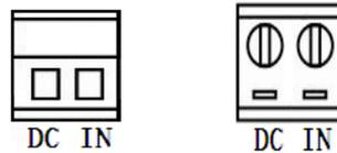
CAN485 interface converter provide DC power input, voltage input is the two terminal form, plug type 2 core spacing of 5.08mm terminals, wherein the power input range of 9 ~ 48VDC. The power support is not polarity that the device can still work normally after the reverse.
