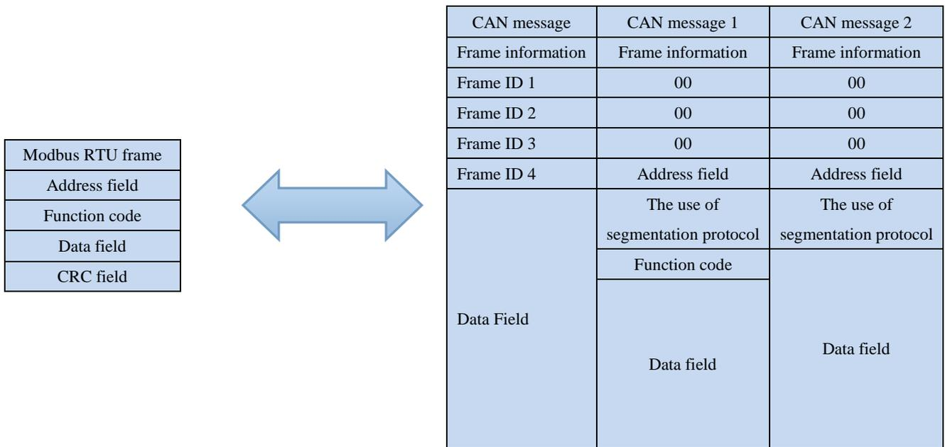
CRC check byte not converted to CAN-Bus message, CAN-Bus message need not check byte with serial frames, because CAN-Bus itself has better check mechanism.
