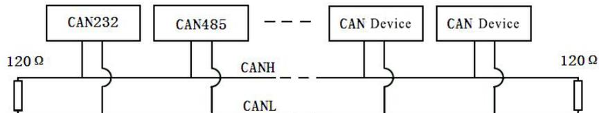
When the CAN485 converter is used as the CAN-Bus network terminal, the two pin is connected to a resistance of 120Ω, otherwise no need to install a 120Ω resistor.
