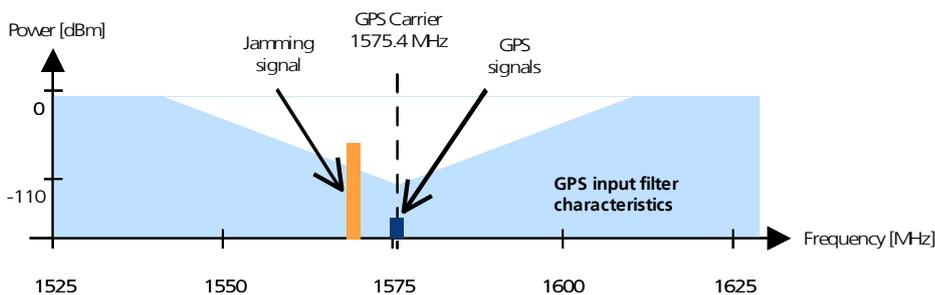
Figure 10: In-band interference signals
