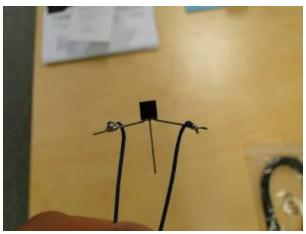
In order for the transistor to switch, the ground of it and the Arduino need to be in common. For this to work, you will need to solder a wire to the ground side of the power supply for the playback module. You will then attach the other side of the wire to the GND connection on the Arduino.
