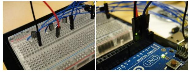
The final step of the build is to connect the transistor's center pins to the Arduino's outputs. I used pins 2 through 5. Just push the center pin into the header on the Arduino at the corresponding pin.
