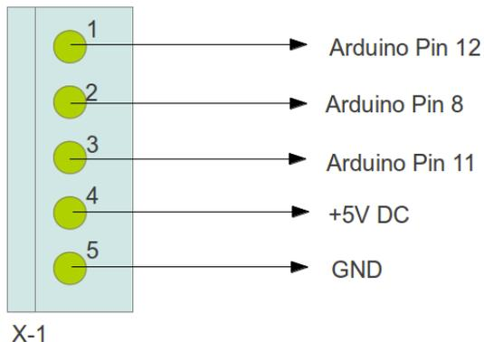
Arduino refers to the controller board running the Electronics123.com, Inc LED Display Controller hex file.
