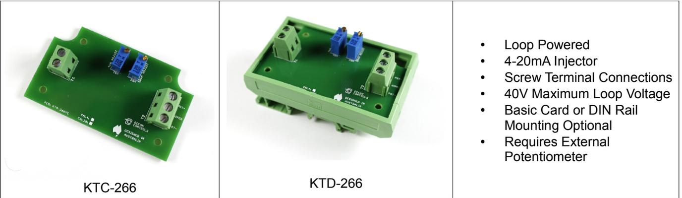
The KTC-266 is a 4-20mA loop powered current calibrator designed to make testing 4-20mA loops simple. With an external potentiometer the KTC-266 and KTD-266 can be used to inject from 4 mA to 20 mA into a current loop. The KTD-266 includes DIN Rail mounting clips.
