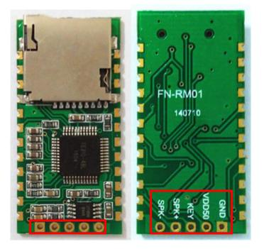
In order to connect to external buttons easily based on AD key control for users to accomplish button control, we made the solder pads at the bottom of the module as shown above marked with the red box. Through AD key function(the pinout "KEY") and connecting with specific values of resistors, users can lead out 5 different functional key control as below. Please refer to the application circuit 5.1 for the connection in details of this part.
