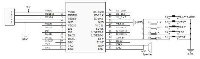
Note: As you can see from the diagram above, except the key Play/Pause that doesn't need a resistor, each key needs a specific value of the resistor.
