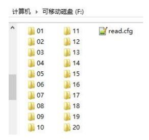
2). Put the sound files in each folder, which can contain maximum 255 sound files. Each folder must contain all Mp3 **OR** Wav audio files. Mp3 and Wav cannot co-exist within each folder. Rename them "001.mp3/wav" to "255.mp3/wav" as shown below. For the quickest timely response once triggered; we suggest that no more than 100 sound files in each folder.
