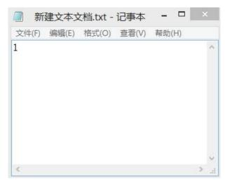
And change the file name "xxx.txt" to "read.cfg" as below, then the configuration file with level hold loop playback mode is made successfully. Please be noted the extension name".txt" of the text file must be changed to ".cfg", otherwise the configuration will not work.
