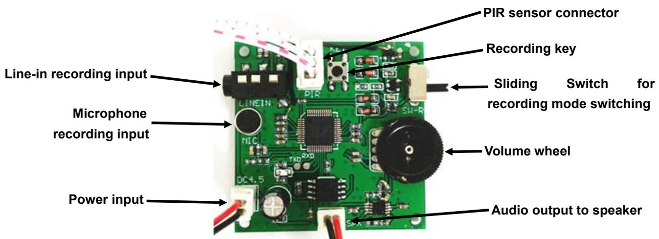
1. Power on the module (be noted that the module itself has no power switch), and wait about 10 seconds initialization.
